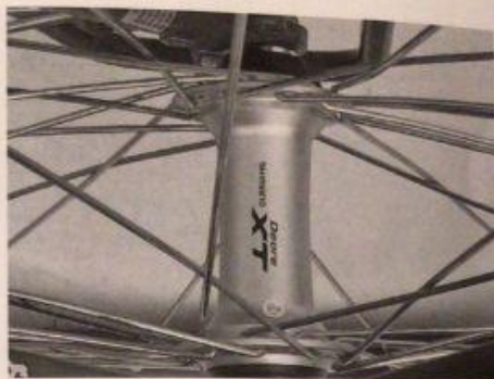
Modern Shimano hub, with large barrel and thin (standard) axle, has great air volume inside. When the hub is cooled, the air inside contracts, sucking in moisture.
