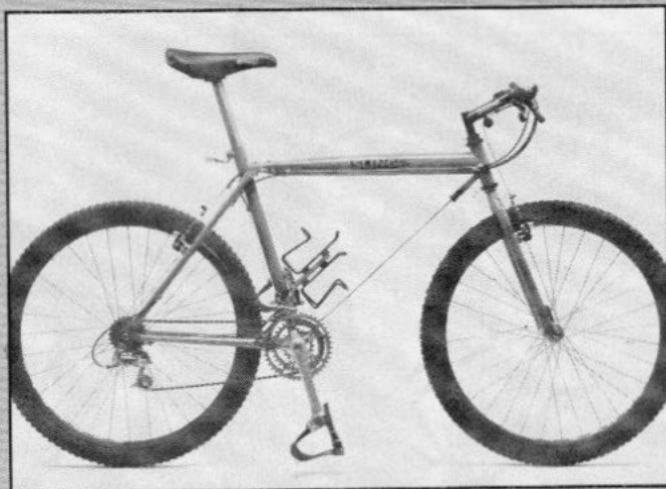
A Scotchply fiberglass spring is housed inside the top tube just ahead of the seat tube. This provides the pivot, and the action is controlled by the spring and cable that replace the down tube. Strange, but effective.
