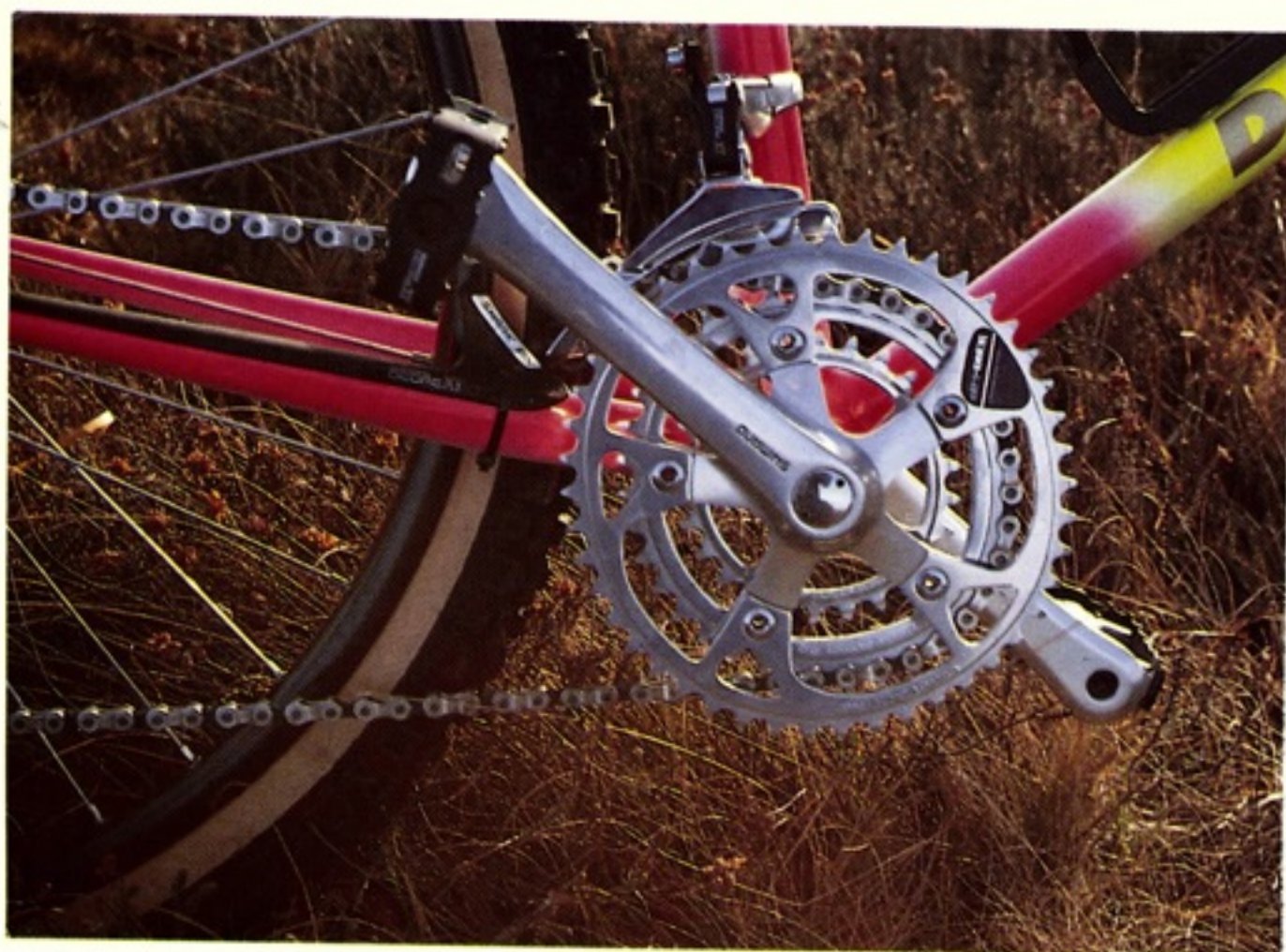
Clockwise from top left: Tioga Prestige bars are very light, colour co-ordinated; Front derailleur cable is routed over the top tube and down the seat tube; Seat cluster with various brazings; Engraved 'D' in the extended seat tube and cables routed along top tube; Deore XT II chainset features new Biopace HP rings; Rear derailleur has Hyperglide and internal cable.
