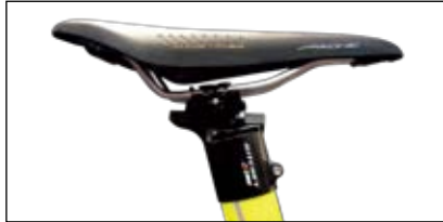
Ritchey WCS custom forged "topper" for the integrated seatmast of the Pro & Team model road bikes
