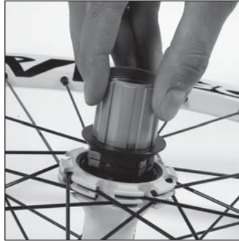
Pull the free wheel body into the hub axle.
