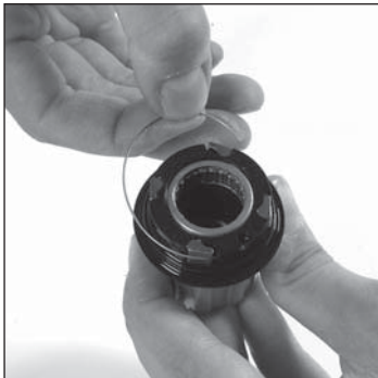
Delicately pull the right hand side of the spring and wind it around the pawl assemblies, ensuring it is correctly positioned at the bottom of the groove.
