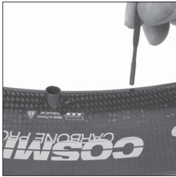
Insert its threaded part into the 1st hole to the right of the valve hole, with the «Made in France» label near you and facing you.
