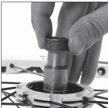
Remove the plain bearing and the spacer by sliding them along the axle.
