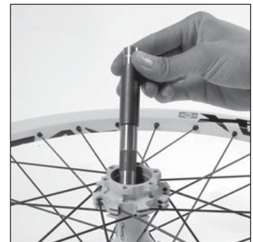
Insert the axle from the non drive side and then refit the non drive side bearing using the assembly tube 324 300 01.
