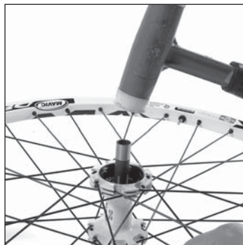
Unclip the fork support nut on the non drive side and then hit the axle on the free wheel side with a mallet to remove the bearing from the non drive side. Repeat the operation for the free wheel side bearing.
