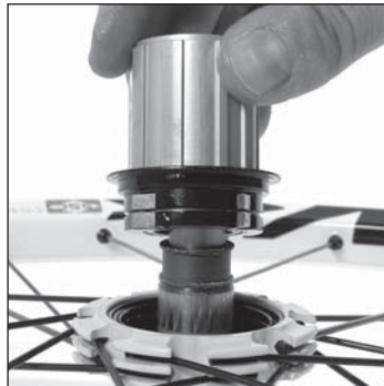
Re-insert the free wheel body into the hub body by pivoting it anti-clockwise.
