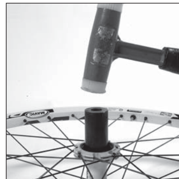
Refit the free wheel side bearing first using the assembly tube 324 300 01. Ensure the bearing is correctly seated in the hub body.
