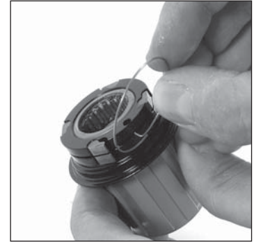
Clean the free wheel body, grease the pawl assemblies and replace them in their housing. Insert the elbowed part of the spring into the insertion hole along the groove.
