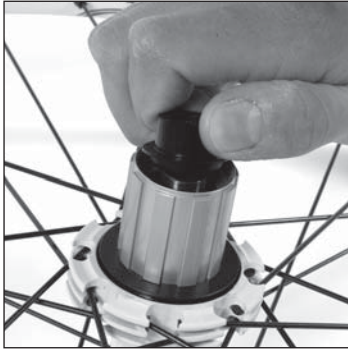
Unclip the fork support nut on the free wheel side.
