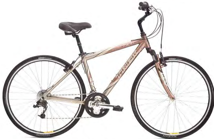
7300™ Frame Alpha Aluminum Front Suspension RST, 50mm Wheelset Alloy front, Shimano RM60 rear hub; Alex rims Crank Bontrager Sport 48/38/28 w/chainring guard Rear Derailleur SRAM X-7 Colors Midnight Blue/Ball Burnished; Matte Latte/Matte Parchment Gold
