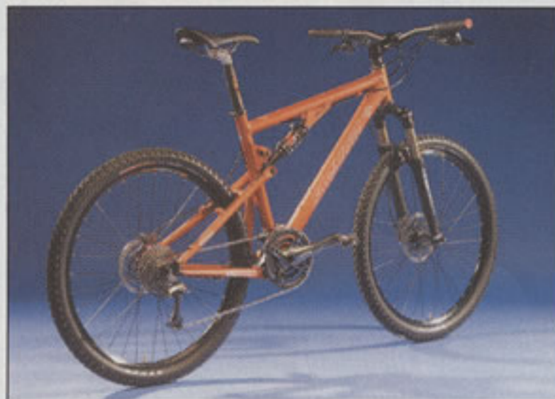
The new kid: The Santa Cruz Blur borrowed something old (the nearly forgotten Virtual Pivot Point rear suspension), revamped it, updated it and served it up as a fresh dish. It tasted so good that it became Santa Cruz's best selling bike.
