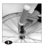
For the front Crossmax™ SL wheel, NEVER replace the bearings on a bare hub. Always replace them when the hub is built into a wheel.
