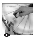
CAUTION : manipulating the integrated nipples greatly affects the spoke tension and consequently the wheel adjustment.
