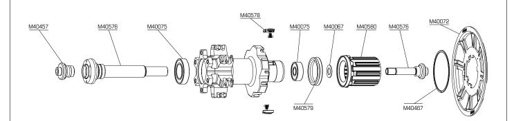
**MAINTENANCE:** Clean with a dry cloth or soap and water. Do not use pressurized water. Caution: The parts on the FTS-L free wheel (pawl assembly, springs, free wheel body) are not compatible with those on the FTS free wheel.
