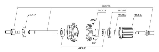
**MAINTENANCE:** Clean with a dry cloth or soap and water. Do not use pressurized water. Caution: The parts on the FTS-L free wheel (pawl assembly, springs, free wheel body) are not compatible with those on the FTS free wheel.
