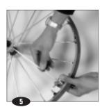
When spokes are missing, the 2 walls can pivot in relationship to each other. However, under the effect of the tension of the spokes, they will go back to their proper position.
