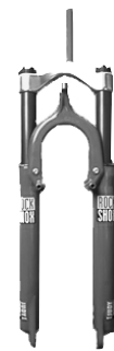
1995JudySL The fork that changed the world! 28mm upper tubes, easy to service cartridge design
