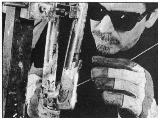
After Joe bends the blades, he dons shades, then brazes up a fork
