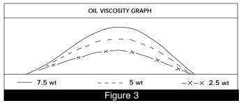
The heavier the fork oil weight, the more damping it will provide. 5-weight Maxima oil is stock in Manitou TPC and TPC Sport forks, but this oil viscosity can be increased or decreased in weight for differing riding conditions and styles.
