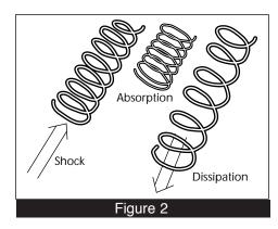
Shock causes the spring to compress and absorb. Rebound occurs as the spring returns, dissipating the energy of the bump.
