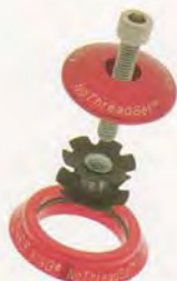
Chris King NoThreadset™ ; for use with threadless steerer tubes. Adjust with a single 5mm hex wrench.
