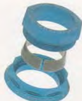
Chris King GripNut™ ; for use with threaded steerer tubes. The unique three piece design has a clamping action that allows it to stay tight even on undersized threads.
