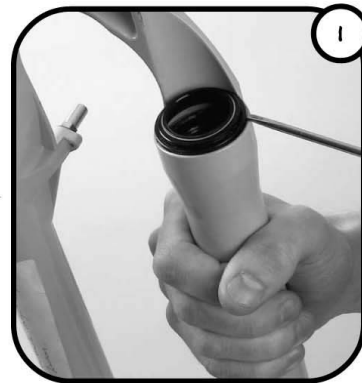
Remove the spring ring with a screwdriver
