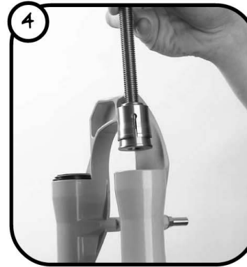
Turn fully clockwise to remove the bushings
