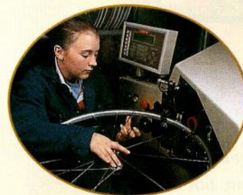
Louise ensures the wheels are laced up properly and tightly to produce a wheel that's up to the high standards set by Dawes.
