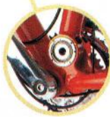
Suspension pivot point with large diameter bearings for maximum rigidity
