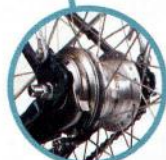
Nexus 7 speed internal hub gear and rear brake
