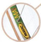
Mavic MA2 36H box section alloy eyelet rims
