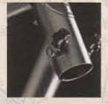
Head Tube Barrel Adjuster: The near-vertical acceptance of ST1 and Ergo shifters has made down tube barrel adjusters obsolete. In response, Merlin now offers lighter, sleeker and more efficient barrel adjusters mounted on the head tube of Extralight, Road and RSR frames.
