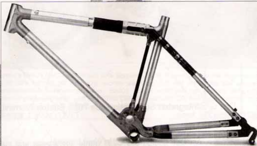
G2-B Integrated Suspension aus Beryllium MMC Be401 (40% Be, 55% Al, 5% Mg) Wert: 50.000,00 DM
