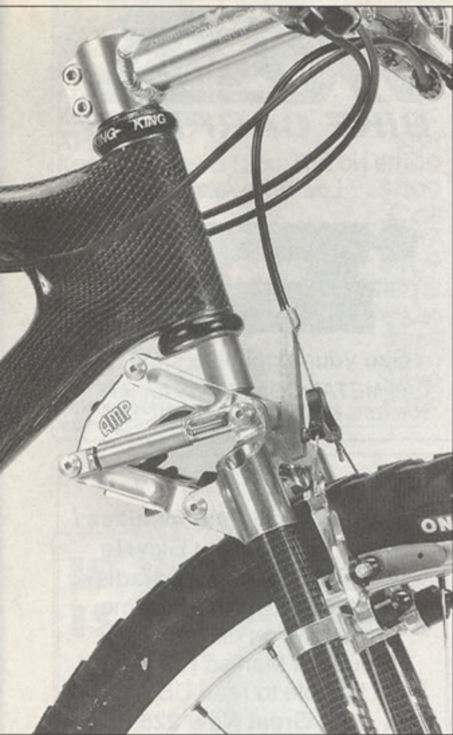
Dream weavers: The High Zoot Talon's frame and fork are turned out in beautiful, clear-coated, carbon fiber. The high-pressure composite molding process that High Zoot uses makes for an ultra-light chassis (unusual for most carbon fiber off-road bikes). AMP's new 2.375" travel fork is far superior to its previous efforts.
