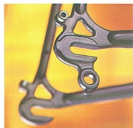
Forged rear drop-outs with mudguard fitting
