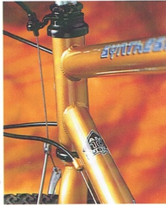
AM-10 tig welded frame
