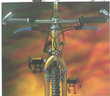
Blue anodised alloy canti-brake system
