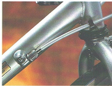
Down tube cable stop/adjuster and guide as featured on Linear, Genesis and Equinox
