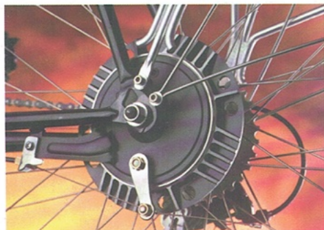
Aria rear drum brake for extra stopping power
