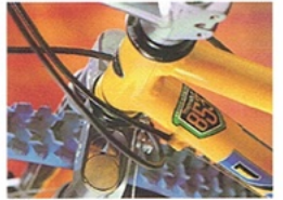
Frame featuring the new Reynolds 853 fillet brazed tube set
