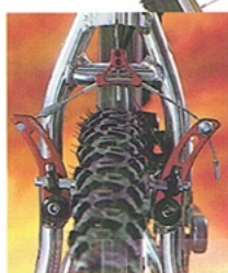
Tektro red anodised canti-brake system
