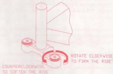
FIGURE 13: FINE TUNING MANITOU EFC
