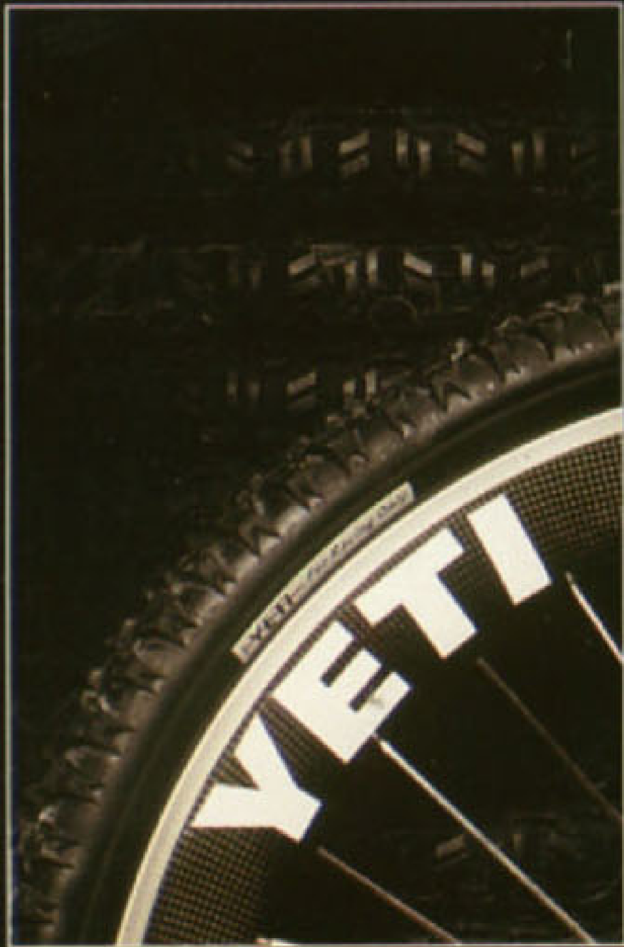
Yeti F.R.O. (For Racing Only) tires. 2.125", Keular beaded, non-directional tread pattern. Great for all conditions!
