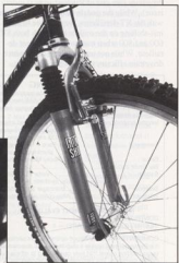
The laterally ultra-stiff RockShox Judy XC complements the resilient ride of the Tange Ultimate Superlight frame.
