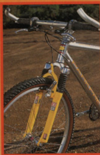
RockShox's Judy SL calms the terrain while Grip Shift X-Ray and Dia-Compe PC-11 levers handle the shifting and stopping duties.
