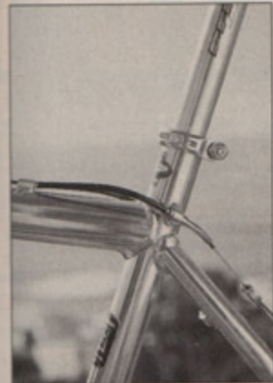
The tube within a ferrule rear brake cable routing seems a bit of overengineering.
