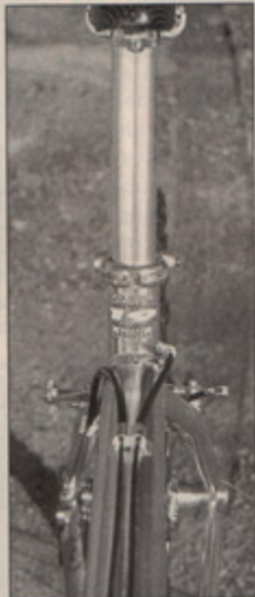
The extended seat tube adds rigidity and leaves no question as to frame size.
