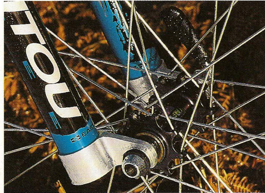
Pulstar straight pull hubs make for strong and stress reduced wheel lacing, but finding replacement spokes can be tricky.
