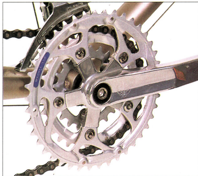
This Sugino-made White Industries crank shares similar features with its £175, made-in-America big brother, but it's not from the same mould. It's forged instead of CNC-machined, heavier by about 50g and doesn't get the high-gloss, polished-by-hand finish. More a cousin than a brother.
