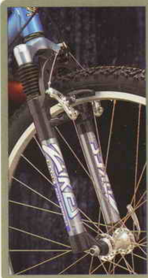
Marzocchi Zokes Elastomer Suspension Weight: 3.0 lbs. Travel: 2 inches
