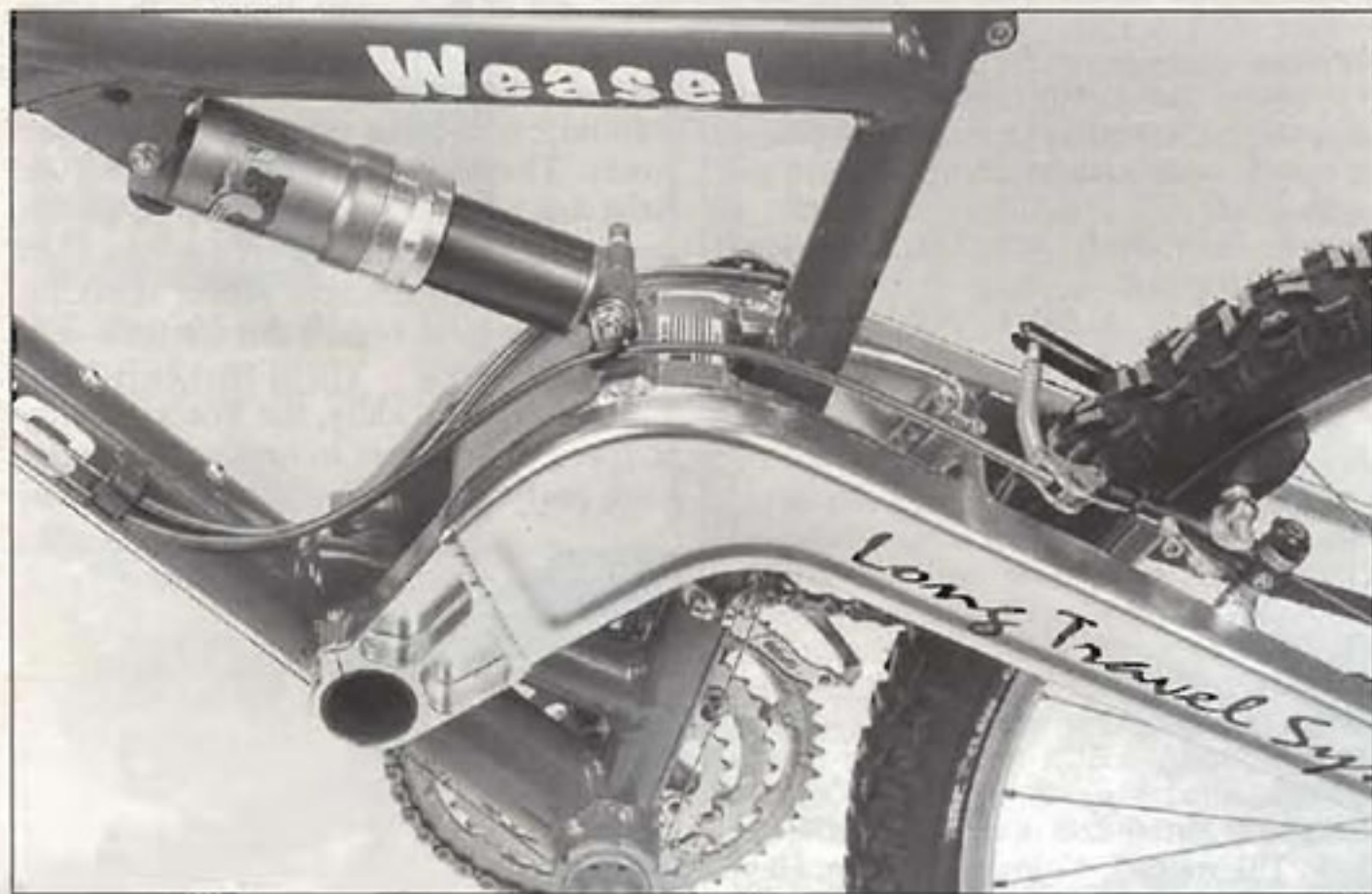
Power-play: While building off-road racing trucks, Brent Foes learned the value of stiff rear suspension and reliable components. The Fox ALPS air/oil damper is the top air shock on the market and uncontested in durability.
