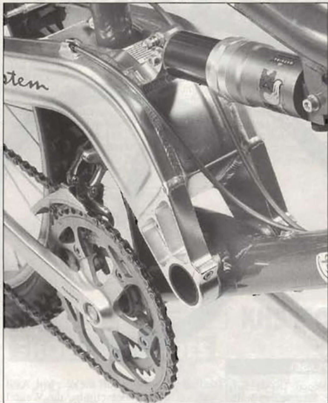
Power-play: While building off-road racing trucks, Brent Foes learned the value of stiff rear suspension and reliable components. The Fox ALPS air/oil damper is the top air shock on the market and uncontested in durability.
