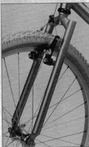
Straight arrow: Fat Chance has been making this fork for a decade (the Big 1). The Fat Chance's performance over moderate bumps was smoother than anyone had imagined possible, due mostly to its supple 1"-diameter tube front end.
