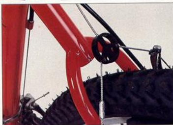
Above: Like Bontrager Fat Chance was one of the first MTB firms to use the wishbone rear end. Consistent with standard wishbone philosophy the Buck Shaver is lightweight, stiff and strong. Trick items on this otherwise 'budget frame' included the Ringle Mojo cable hangers.
