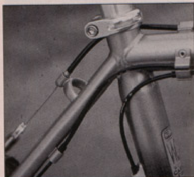
Notice the taper of the seat tube, the riveted cable stops and the rather clean welds.
