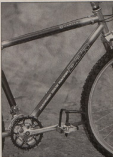
The DBR welded carbon-fiber frameset combines the weight savings and stiffness of a composite with the ease of assembly and versatility of TIG-welded chrome-moly joints.
