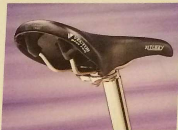
▼ Ritchey Vector saddle with Cr-Mo rails & leather cover
