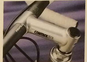
▼ Control Tech alloy stem; Tioga Master DLS headset; 100% alloy construction
