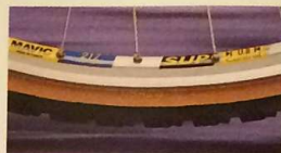
▼ Mavic 217 S.U.P. + U.B. control rims with eyelets; Perfect S.U.P. sides for performance brake control
