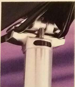
▼ Avenir light alloy seat post with "Dial-Adjust"
