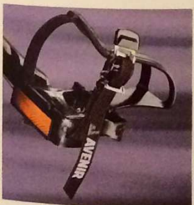
▼ Resin pedals with toe clips and straps
