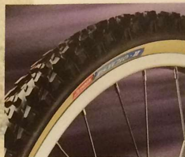
▼ Aggressive tread Tioga Psycho II tires; Weinmann 4019 alloy rims, fully brushed for improved braking;
