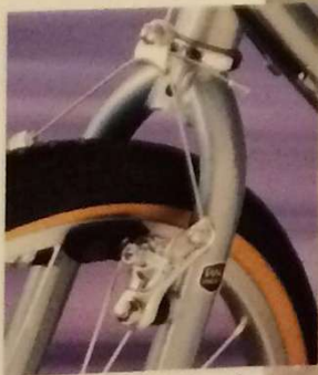
▼ Tange Unicrown high tensile steel fork with ovalized blades for increased durability
