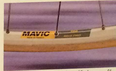
▼ Mavic 195 alloy rims with modified aero profile
