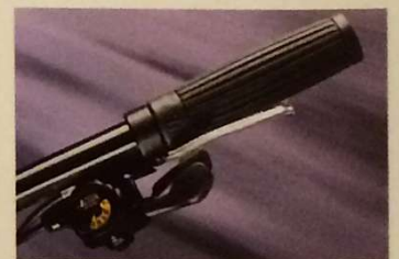
▼ Shimano C-90 Rapid fire TX shifters with optical gear display
