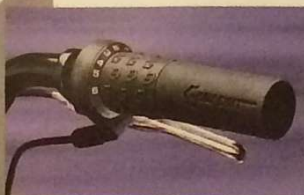
▼ 21 speed Grip Shift MRX-100 with gear indicator
