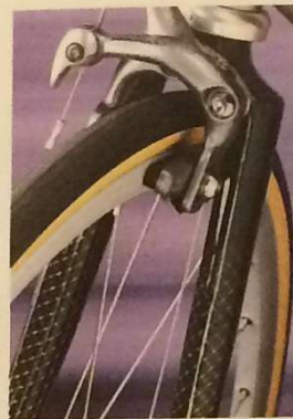
▼ New Diamond Back alloy/carbon fork; Aluminum core with carbon fibre; Chromoly steerer tube
