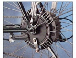
Arai drum rear brake for assured stopping power.
