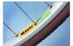
Mavic tandem 40 hole anodised rims for perfect balance, strength and lightness.
