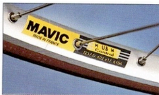
Mavic T237D box section double eyeletted rims with new 'UB' control for improved braking performance.
