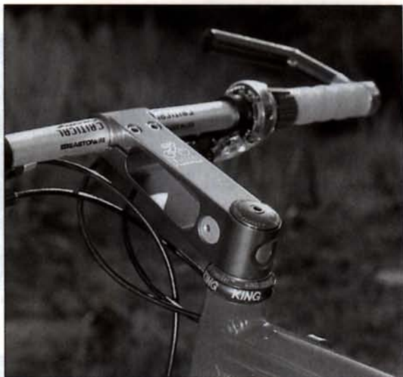
Grip Shift X-Ray shifters let you find your gear, and Critical Racing's see-through stem helps eliminate control-center flex.
