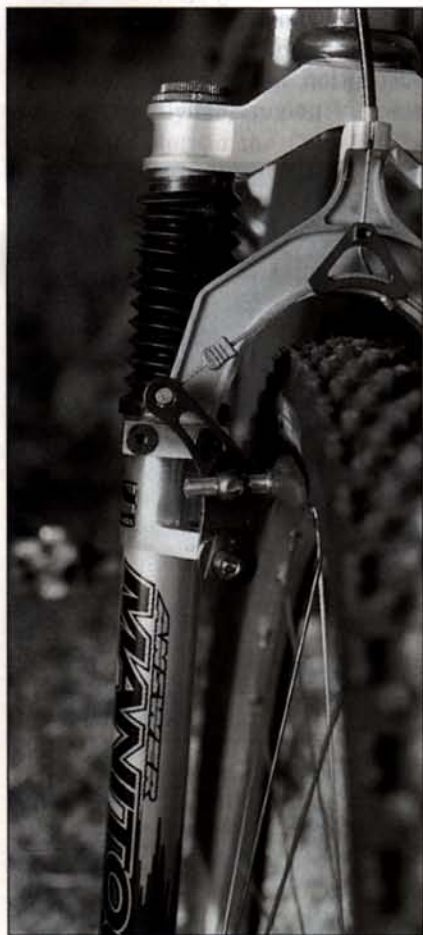
Critical Racing cantilevers mounted with Aztec pads provided excellent braking power.
