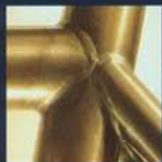
Sequential Tungsten Inert Gas (TIG) welding eliminates heat distortion and maintains precise joint alignment.
