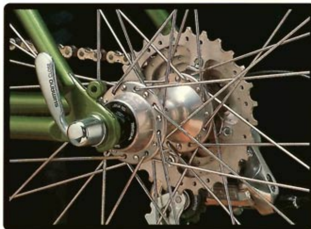
Shimano quick release hub. Please ask your dealer to show you how it works.
