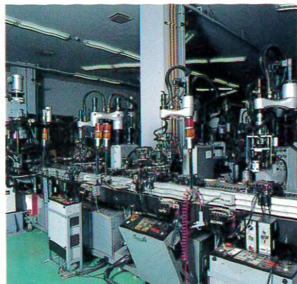
Robotic assembly line.
