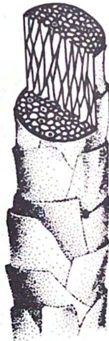
A WOOL FIBER HAS OVERLAPPING SCALES THAT TRAP DIRT NEAR THE SURFACE, WHERE IT IS EASILY WASHED OUT.
