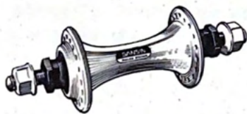
DA BUB HUB: SANSIN (JAPANESE) ALUMINUM, WITH THEFT-DISOURAGING NUTS.
