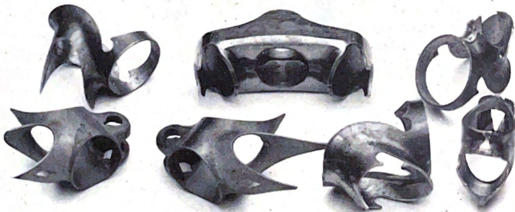
AN ASSORTMENT OF STAMPED LUGS FROM FRANCE, AND AN INEXPENSIVE STAMPED FORK CROWN FROM JAPAN.
