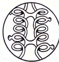
EACH WOOL FIBER HAS A SPIRALING CRIMP WHICH LETS IT STRETCH, THEN SPRING BACK.
