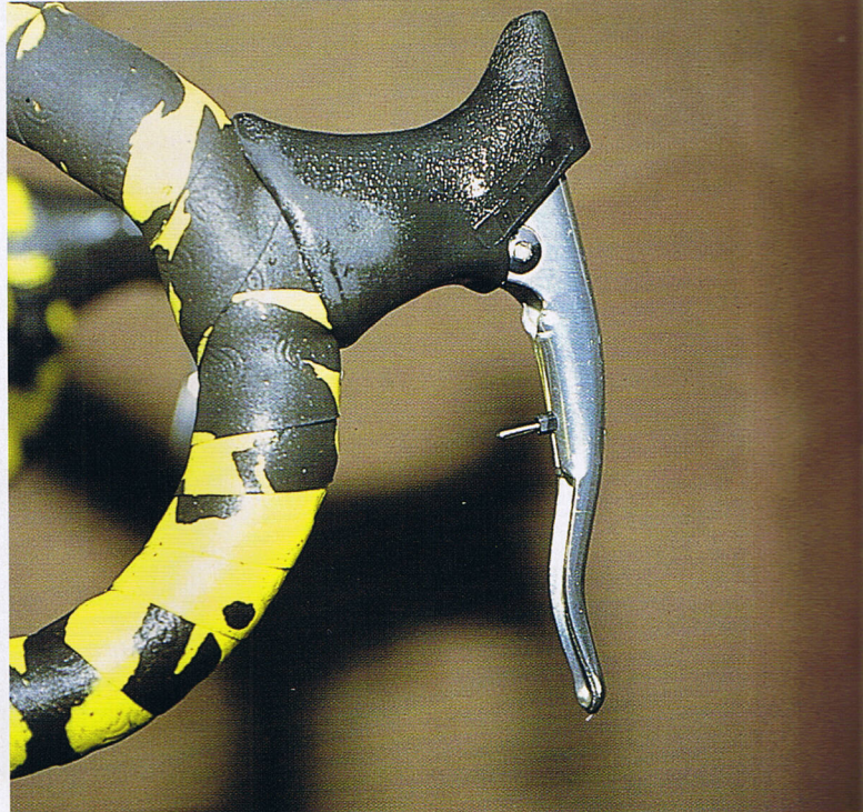
Above and below: with two switches built into the Zap system, it is possible to change gears whether riding on the tops or the drops. The battery powering the set-up is hidden inside the bars.
