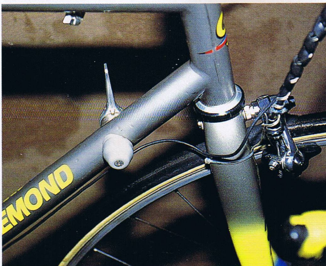
Welds on the titanium frame are cleanly and smoothly executed — and the Zap wiring adds to the sleek appearance.
