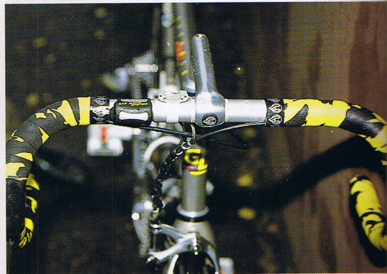
Above and below: with two switches built into the Zap system, it is possible to change gears whether riding on the tops or the drops. The battery powering the set-up is hidden inside the bars.
