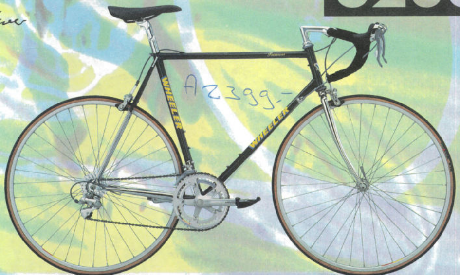
Group: SHIMANO 105 SC, 16SP DUAL CONTROL LEVER Frame: TANGE INFINITY DOUBLE BUTTED CR-MO INVESTMENT CAST LUGS Color: PERL DUNKEL GRÜN
