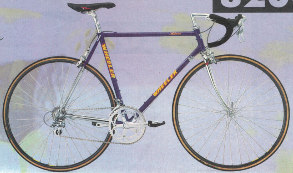
Group: SHIMANO DURA ACE, 16SP DUAL CONTROL LEVER Frame: SILVER BRAZED TANGE PRESTIGE, INVESTMENT CAST LUGS Color: CHROM PURPLE
