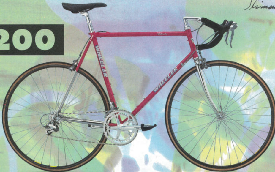
Group: SHIMANO ULTEGRA, 16SP DUAL CONTROL LEVER Frame: TANGE No 2 DOUBLE BUTTED CR-MO INVESTMENT CAST LUGS Color: PERL MAGENTA
