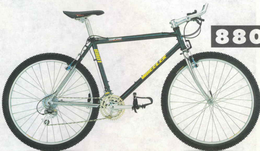
Group: SUNTOUR XC-PRO MICRO DRIVE, 24SP ACCU SHIFT Frame: LUGGED TANGE ULTIMATE PRESTIGE, SILVER BRAZED, ALU BAR-STEM COMBO Weight: 11,4 KG Color: CHROM DUNKEL GRÜN
