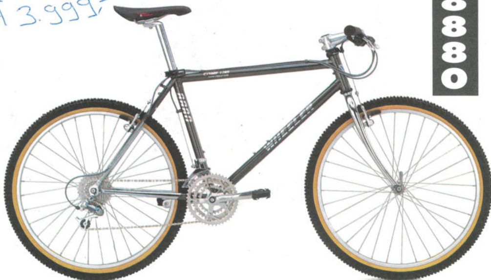
Group: SHIMANO XTR, 24 SP STI PLUS Frame: LUGGED TANGE ULTIMATE PRESTIGE, SILVER BRAZED, ALU BAR-STEM COMBO Weight: 11,2 KG Color: CHROM GRAU
