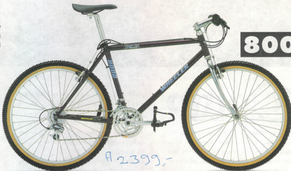
Group: SHIMANO DEORE XT, 21 SP STI PLUS Frame: LUGGED TANGE O.S. DOUBLE BUTTED CR-MO CYNCH STEERING SYSTEM Color: CHROM MAGENTA
