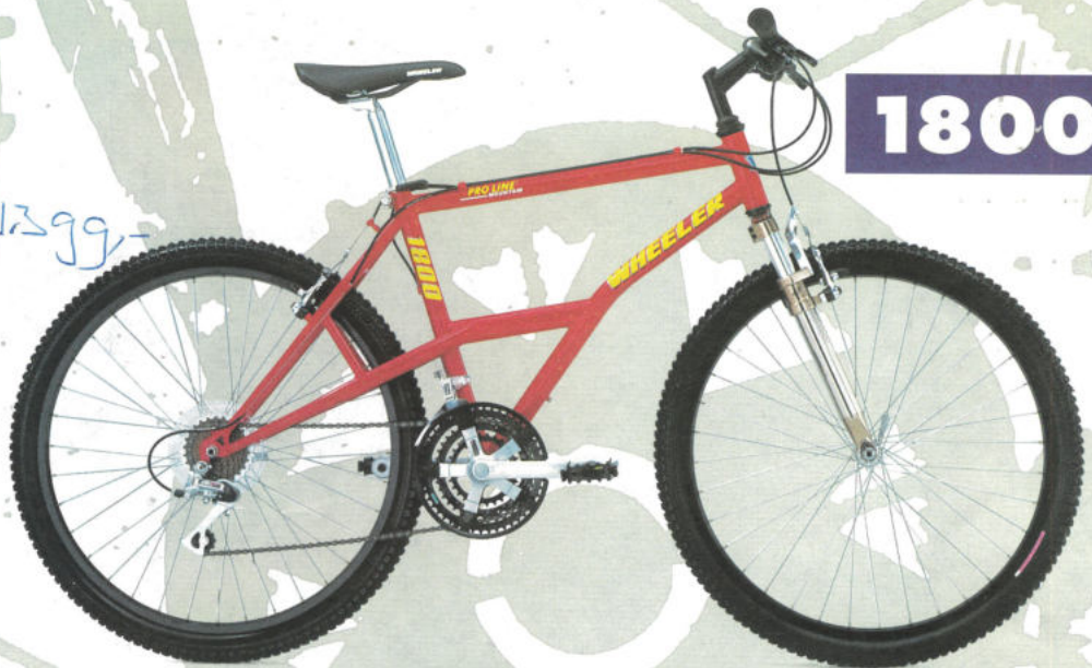
Group: SHIMANO ALTUS C10, 21 SP STI RAPID FIRE Frame: T.I.G. TANGE O.S. CR-MO, ELEVATED STAYS Fork: POLYGON SUSPENSION FORK Color: ROT
