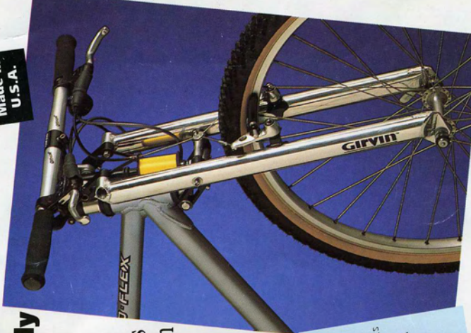
The Girvin Fork's curved axle path requires a slight initial backward travel in line with the bump force, before resuming a more conventional vertical movement.
