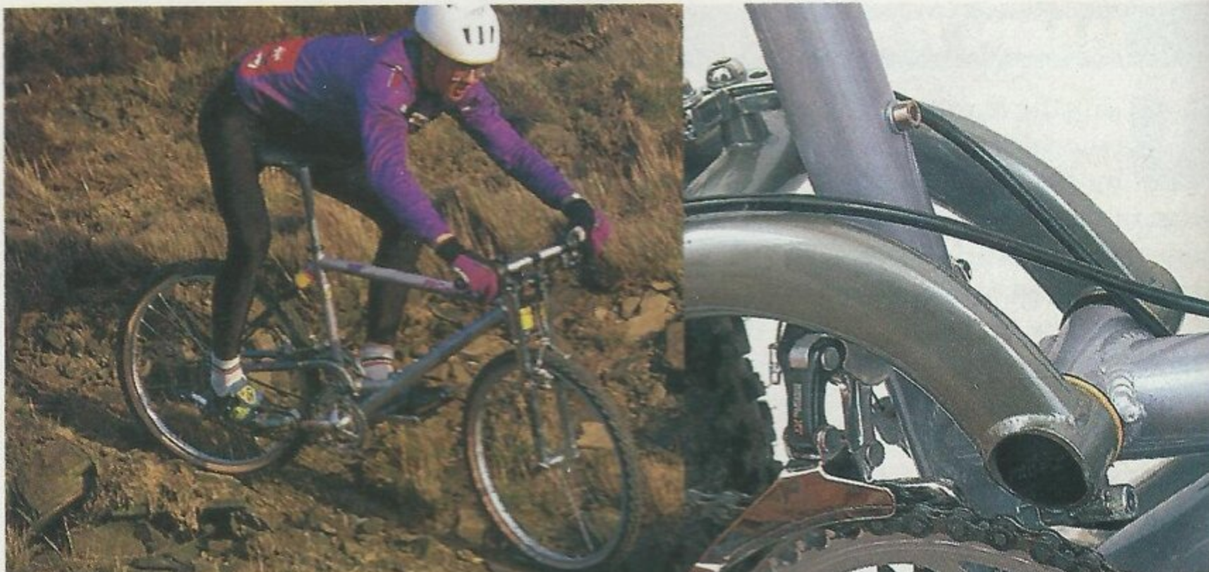
Offroad's vast experience in suspension bikes shows in the sophisticated yet simple design of the 953. Offroad's pivot has lowered over the years, making for a very active back end.
