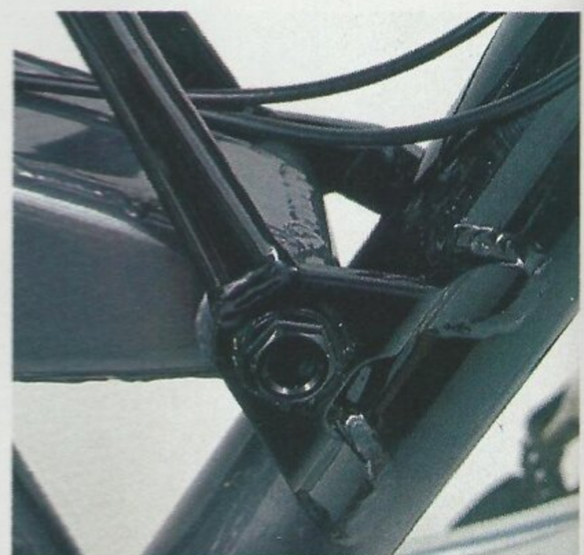
The highish pivot means some lock-out under hard pedalling, but it works most of the time.
