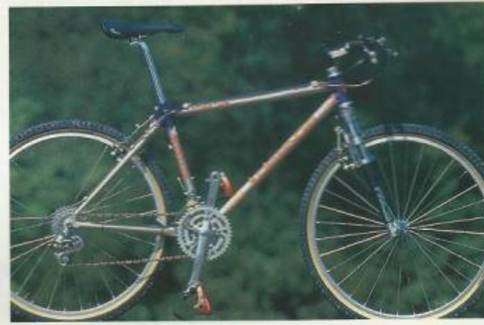
Left: the front hub is a Hope titanium instead of the more usually supplied XC Expert...
