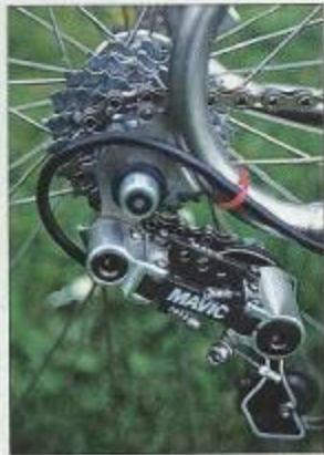
A Mavic mech perforated and adjusted for 11-23T 700-CX Shimano hybrid micro gearing.
