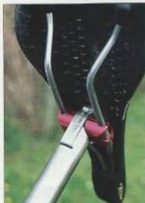
The titanium seatpin is home-crafted. A jubilee clip replaces the seat clamp bolt - how long it will last we don't know.
