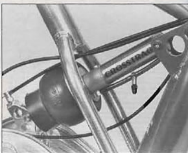
The blimp: A Firestone air bladder provides the springing for the oil-damped hydraulic shock absorber. Crosstrac uses crossover air lines with Presta valves for adjustment. Thankfully, air pressures are low enough to change on the trail without a nitrogen tank.
