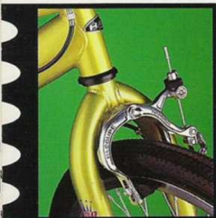
Dia-Compe 883 Nippon front brake. Combined with Dia-Compe AD 990 U-brake in the rear and chrome-plated rims, the 1993 Master has burly stopping power plus.
