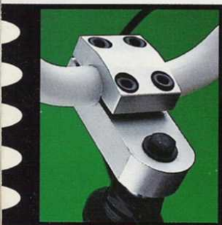
Fusion precision-machined aluminum billet stem. Low-profile motocross handlebars.
