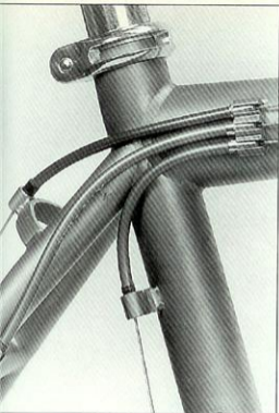
Three versions: Diamond Back is making their titanium frame available either as a frameset, or complete with a Shimano LX/XT gruppo, or with a Shimano XTR gruppo. Manufactured by Sandvik, the bike has many design features, like the ovalized top tube, seat tube and tapered chainstays that are custom for the Diamond Back Racing group.
