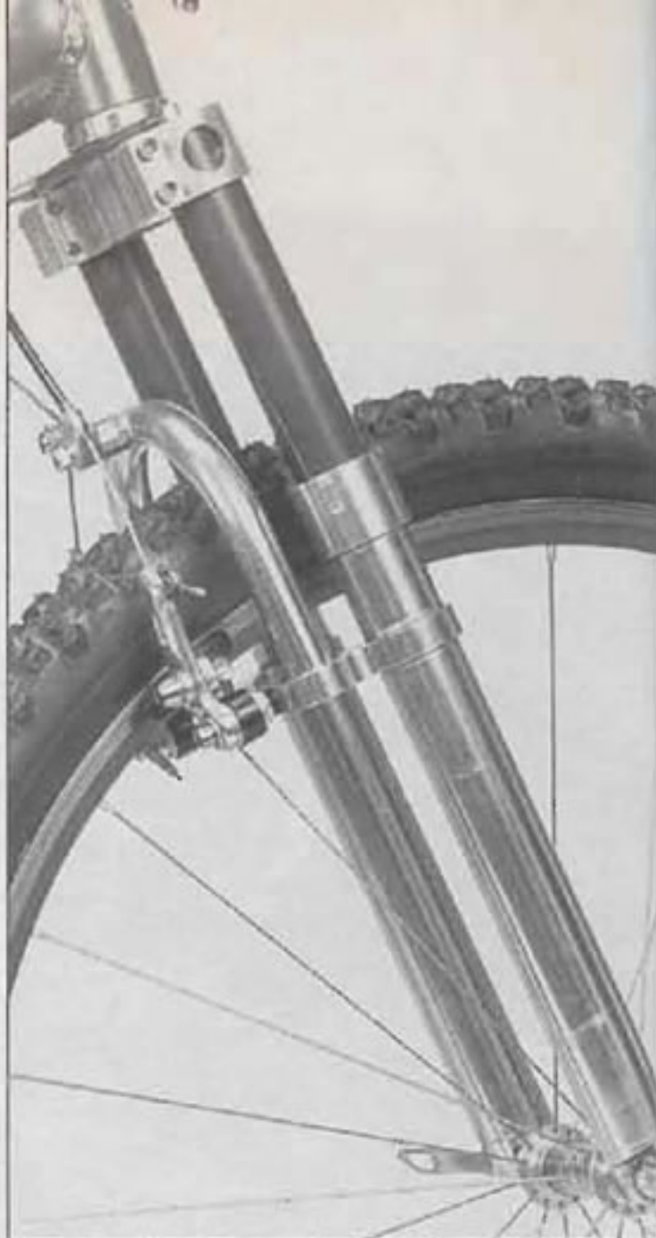
Big bump eater: Hard-anodized aluminum fork legs guide the polished alloy legs across 4" of incredibly plush travel. The fork brace and cantilevers are mounted on the back of the forks to take advantage of the rotational inertia of the front wheel.
