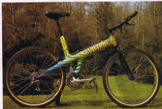
The Trimble's unique looks come from its one-piece 'monocoque' construction. It's tough, light and comfortable.
