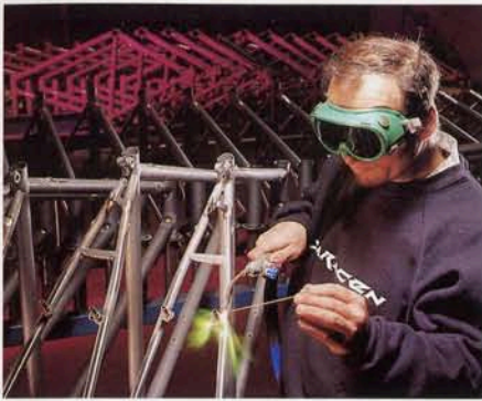
Hand-finishing of the frame - from fitting a full complement of neat braze-ons to finishing the frame ready for painting - is typical of the attention to detail we lavish on our bikes before they leave the factory.
