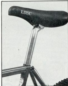
The seat clamp is a Ritecye trademark, and a great area to show off the fillet-brazed welds. Note how the rear brake cable routes over the top of the clamp, and that it's not a stop, but a guide. It's different, but it works.
