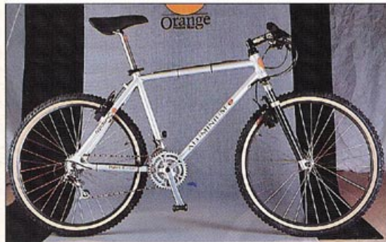
◀ Aluminium 'O' with Suntour XC Comp Microdrive, Pace RC35 Forks, Magura Hydrostope and SPD pedals
