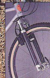
▲ Pace Suspension Forks with Magura Hydraulic Brakes
